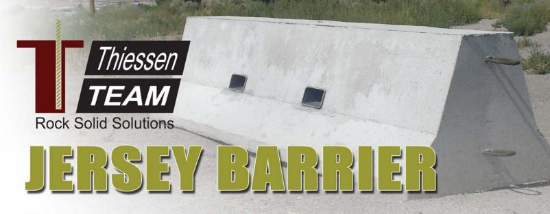
The Thiessen Team Jersey Barrier is designed for mining applications. Steel re-enforced core, structural fiber re-enforced concrete and a wider base for stability, is the make-up characteristics for the Thiessen Team Jersey Barrier to meet any required demand.
